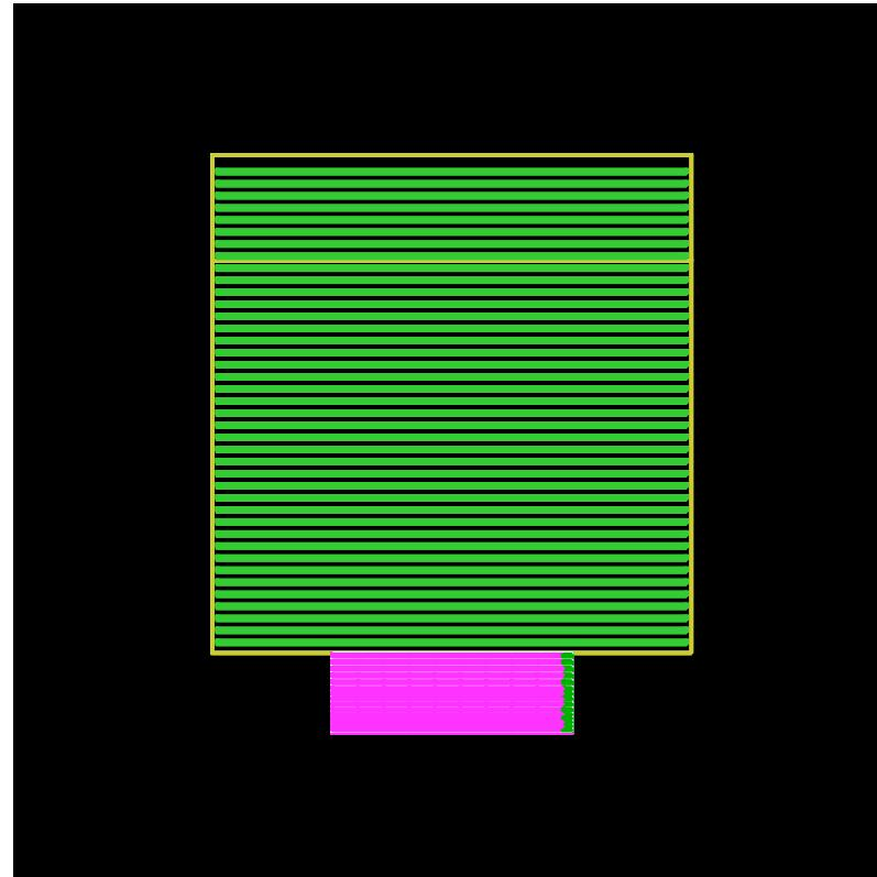
**ECAL** 30 layers  $\times$  50 cm  $\times$  38 cm interleaved with 0.5 mm Si pads
