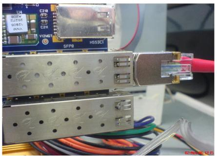
The transceiver inserted into the cage on the FPGA board.
