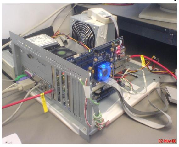
The test stand used for initial development. The FPGA card is installed in the machine, and there is a PClexpress Gigabit Ethernet card installed.
