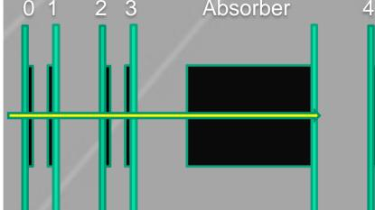
Absorber constructed of multiple slabs of 3mm thick Tungsten (6/7  $\chi_0$ ) kept constant distance from rear sensors. (beam arrives from left)
