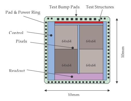
Four pixel variants with shared control and readout circuits so the device behaves as a single sensor.
