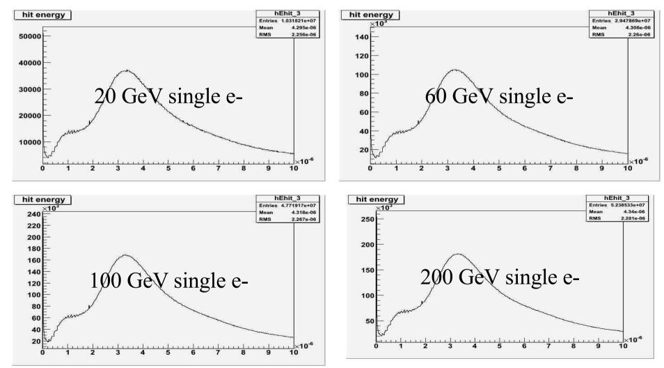
Mean value dose not depend on incoming electron energies. --->Single MIP in each cell. (Individual MIP can be detected.)
