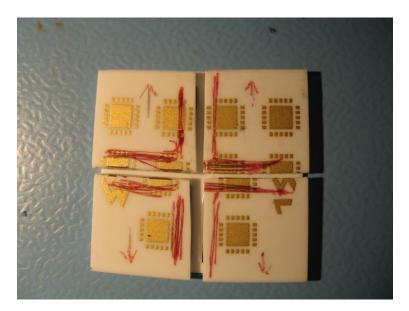
To the top of each chip a drop of epoxy was applied on one side, and a 10 x 10mm ceramic placed on top.
