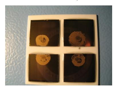
It can be seen that in every case, the glue remained on the chip, and no glue remained on the small ceramics.
