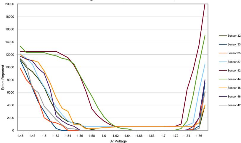
Configuration errors; VDD1V8SRAM sweep
