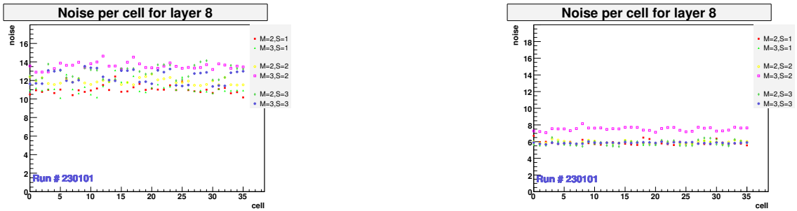
Figure 18: Layer 8, mean noise observed per wafer before any corrections, and after all corrections
