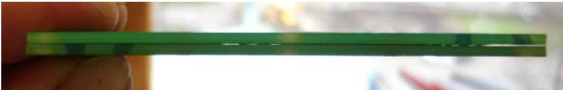
Figure 8: Side view of two glue-test PCBs bonded with conductive glue. The spacing is 100\mu\text{m} .
