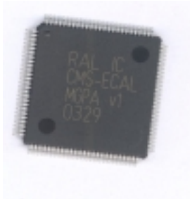
Figure 5. MGPA chip in 100 pin TQFP package
