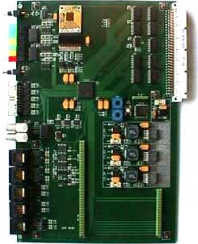
Figure 4: The 6U VME APV25 Emulator card. The APV25 ASIC can be seen mounted on a copper PCB at the top. The FMM inputs and TCS outputs are seen at the lower left side.
