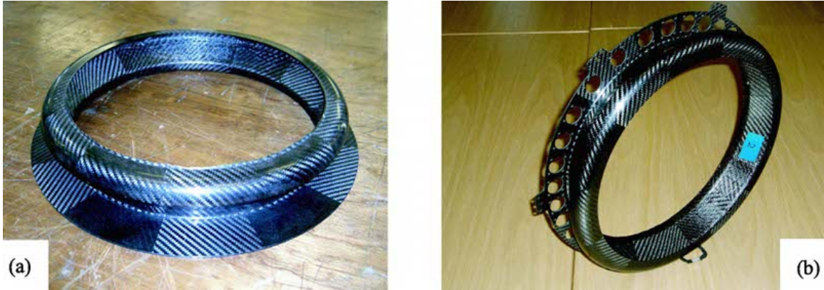
Figure 6: (a) Photograph of a carbon fibre station body after curing in the autoclave. (b) Photograph of the station body after final machining. The holes that take the station connectors and the flanges that mate to the space frame are shown.
