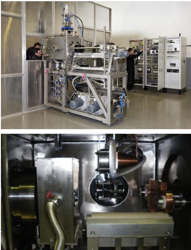
Figure 2: Upper frame: Overview of the installation: Faraday cage, diagnostics vessel, power supplies. Bottom Frame: From left to right Quadrupole, Dipole, Faraday Cup, RPA (behind) and Pepperpot grid.
